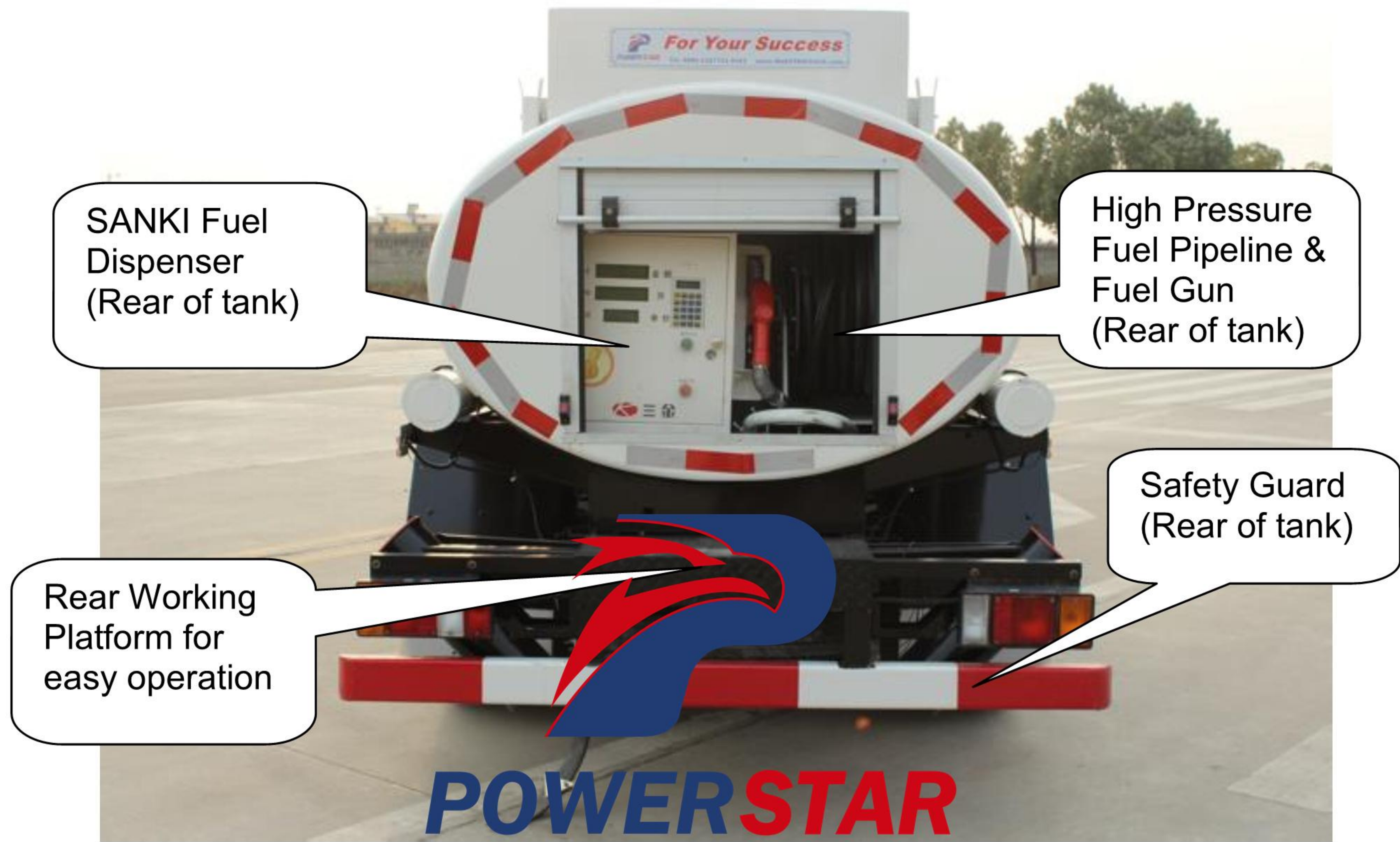
Rear of the Tank: Working Platform, SANKI Fuel Dispenser & Pipeline Container
